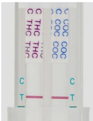
Fig. 4 Example of Invalid Test Results
