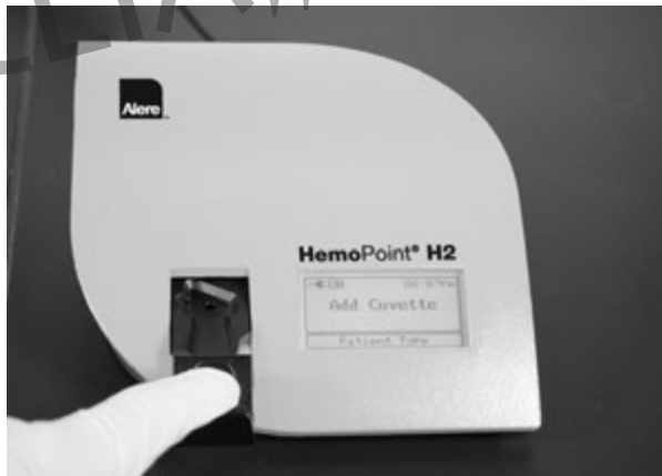
Illustration 16: Opening the Alere HemoPoint® H2 Microcuvette holder.
