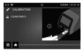
Sofia 2 indicates when the Calibration Check is completed, ♥ or ⊗. Select ♠ to return to the Run Test screen.
