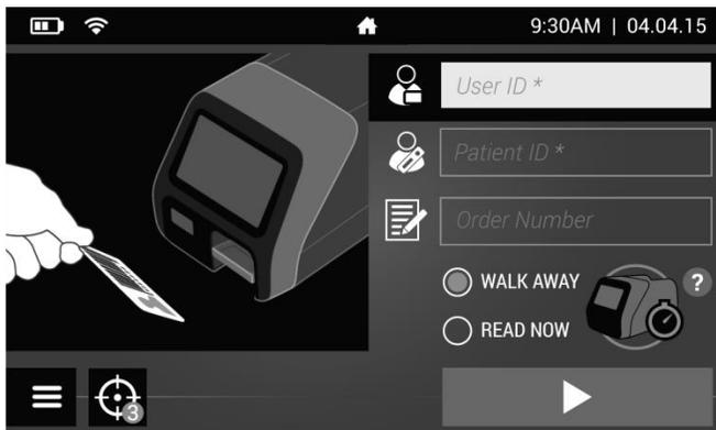
2. If necessary, input the Patient ID and Order #, if applicable, using the barcode scanner or manually enter the data using the touchscreen.
