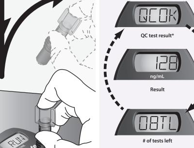
This result cycle remains displayed for 15 minutes or until the next Test Cartridge is inserted.
