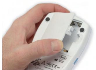
Open the battery compartment on the back of the meter.
