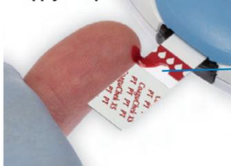
Find the target area on the test strip. You can dose from the side or top.
