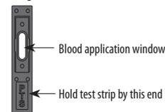
3. When APPLY SAMPLE appears on the display, use a capillary blood collector or pipet to apply 35-40 µL of whole blood to the test strip blood application window.
