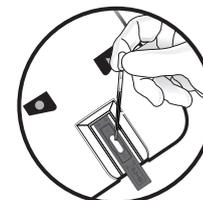
4. In as little as 90 seconds, the results will appear on the display automatically on the analyzer. As necessary, press NEXT to view additional results. Remove and discard test strip. Do not add more blood to a test strip that has been used.
