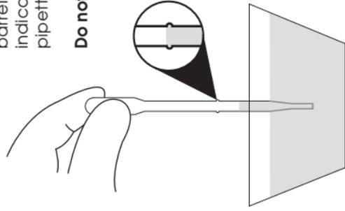
Expel **entire** contents of the barrel into the sample well of the test device. No drop counting required.
