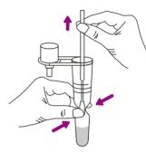
10 CLOSE the dropper cap firmly that is attached to the buffer tube.
