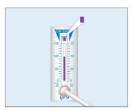
► Start timing and note activation time. ► After 2 minutes, but not longer than 5 minutes read alcohol concentration at the highest point of the purple bar. The QA Spot must be purple. ► Show result to donor.
