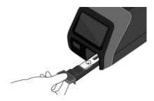
5. Sofia 2 will start automatically and display the progress, as shown in the example below. In WALK AWAY Mode, the test results will be displayed on the screen in 15 minutes. In READ NOW Mode, the test results will be displayed on the screen within 1 minute. See Sofia 2 Interpretation of Results section.
