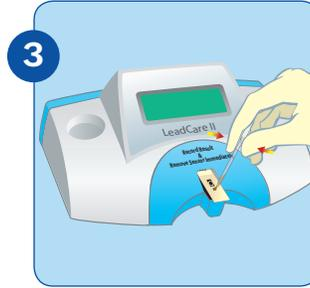
**3 Test:** Place a drop of sample on the sensor; results in 3 minutes.
