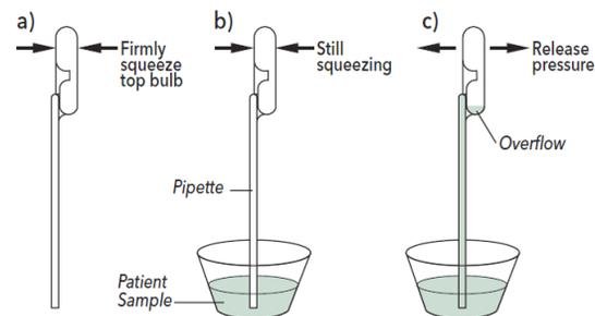
\*Note: The pipette is designed to collect and dispense the correct amount of liquid sample.
