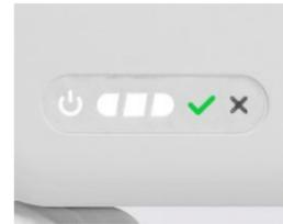
**C.** Wait approximately **28 minutes** for a green check mark to appear indicating the test is finished running. **Note:** If a **red X** appears at any point, stop, do not read test results, and retest.
