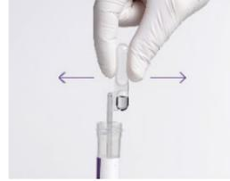
**C.** Release the upper bulb **slowly** to fill the shaft. Keep pipette tip submerged until shaft is full. Extra fluid should enter the lower bulb.
