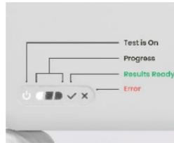
**B.** Check that the first progress **indicator light is blinking**. Lights will initially blink and then become stable as the test progresses.
