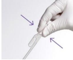
**B.** Squeeze the **upper bulb** of the provided pipette and submerge the tip to the **bottom** of the sample tube.
