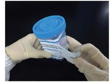
4. At 5 minutes, peel the label and read results. Do not read after 60 minutes.
