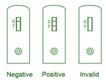
Negative: At five minutes, one rose-pink color band appears in the control (C) zone indicating a negative result and that the specimen does not contain a detectable level of human hemoglobin.
