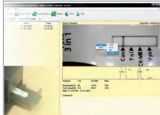
Quantitative results by Nano-Checker 710 are automatically determined and displayed or printed as PDF format report.
