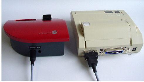
Illustration 33: Connecting the Seiko DPU-414 printer.
